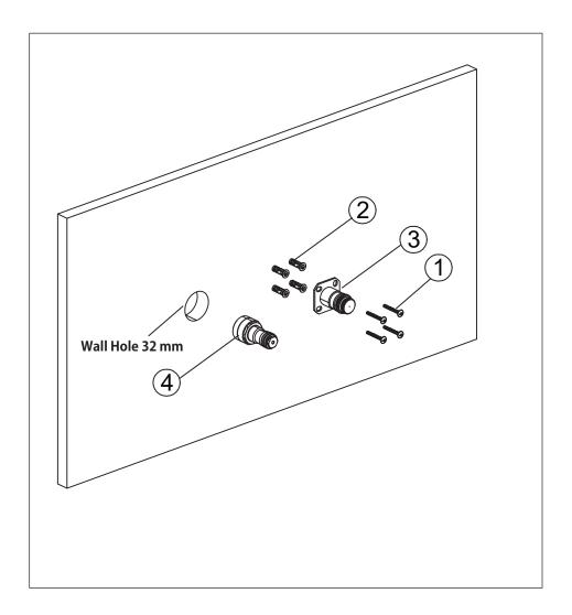
Secure the mounting seat (3) using screws (1) and wall plugs (2). Thread the female 1/2" NPT adaptor (4) onto the wall.
