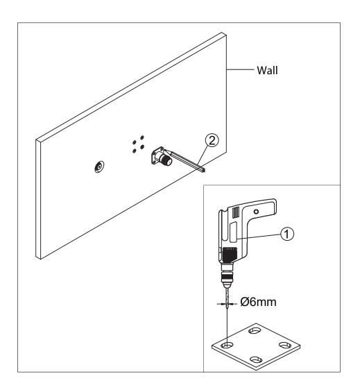
Mark the locations for the screws (1) and then drill the four holes [6mm diameter] for the screws (2)
