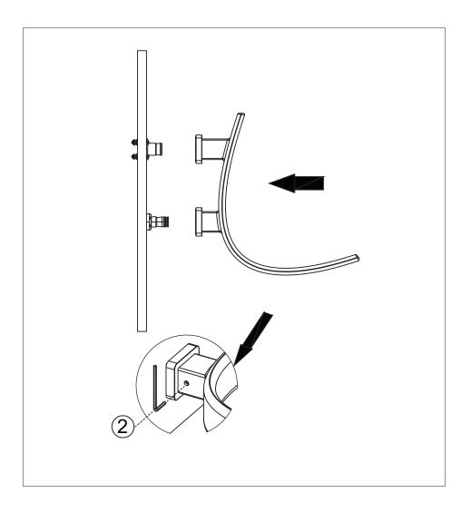
Loosen the hex screws (2) from the faucet with an allen wrench. Loosen the same screws on the opposite side in the same way.
