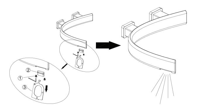
IMPORTANT: After installation is complete, loosen the set screw (1) with Phillip's screwdriver, then remove aerator (2) with aerator wrench (3) provided to flush the water lines and check for leaks. If you discover any leaks, check your connections to ensure they are installed properly and reinstall the aerator.
